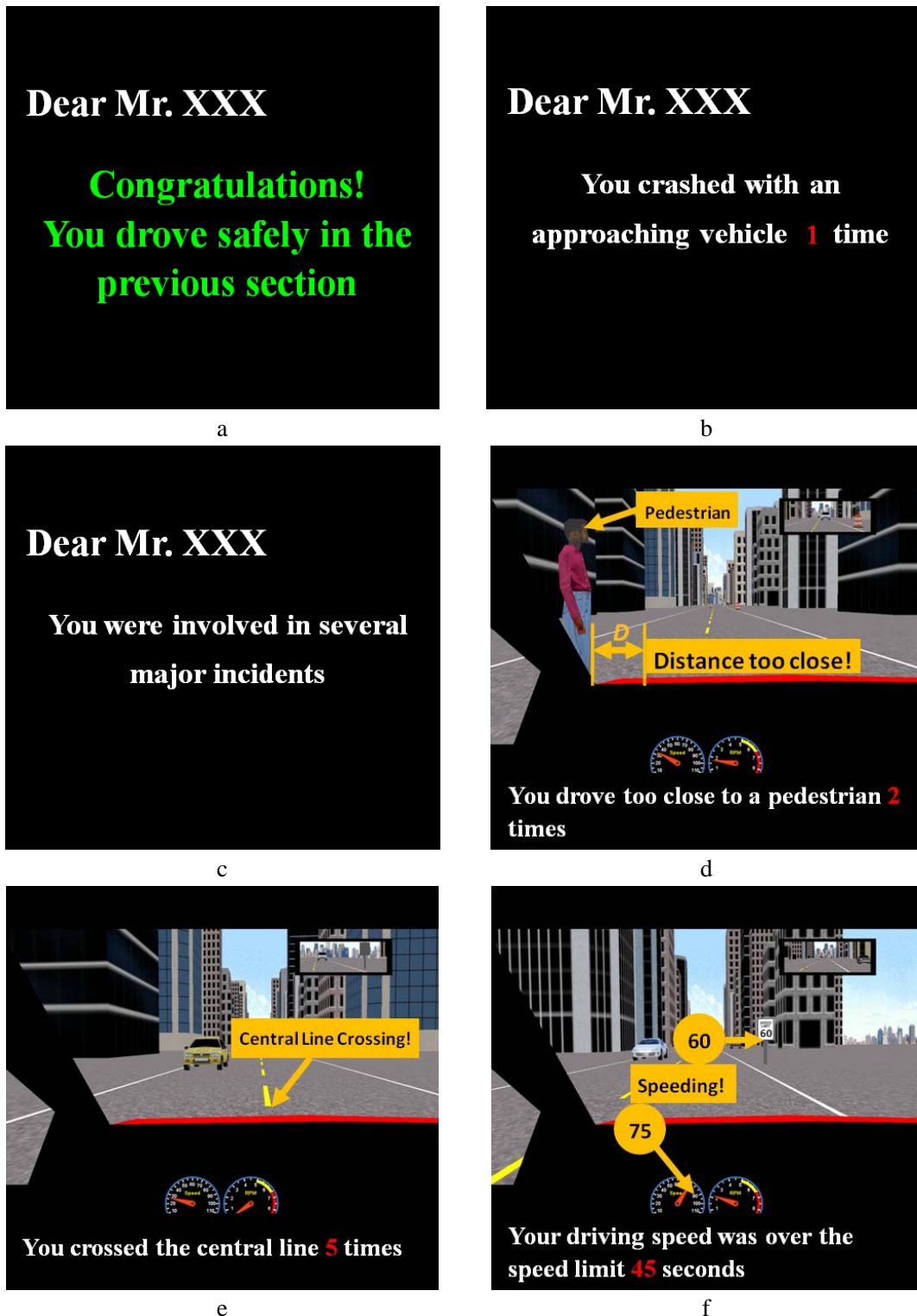
Fig. 1. Samples of the trip report (a. Positive feedback for no accidents or incidents; b. Information on accidents; c. Information on major incidents; d. Information on the frequency of driving too close to a pedestrian; e. Information on central-line crossing frequency; f. Information on speeding duration)
